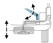
Note: Do not stow the full size tire or any flat tire under the vehicle.
